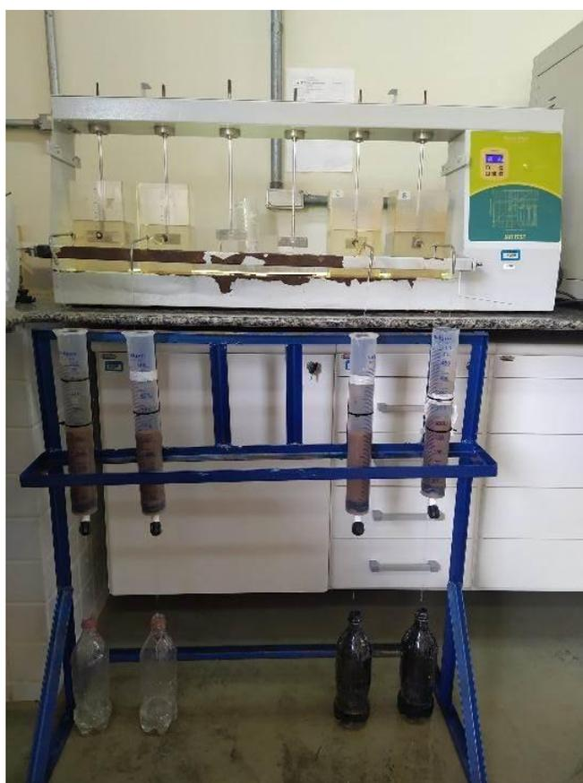
**Figure 3.** Jar-test equipment associated with filters.
