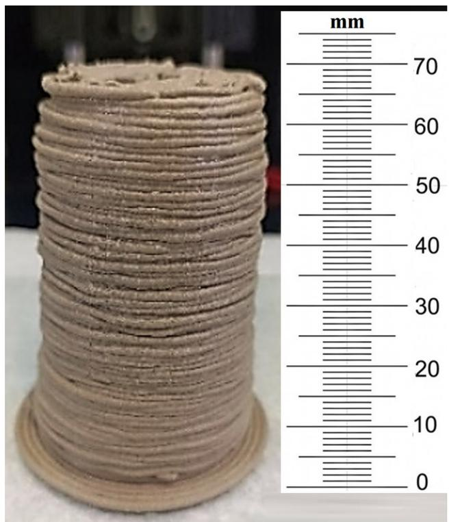
Figure 8: Image of cylindric geopolymer sample printed using metakaolin from batch 2, 0.05% of PP fibers, and 7.46 M alkaline solution.
