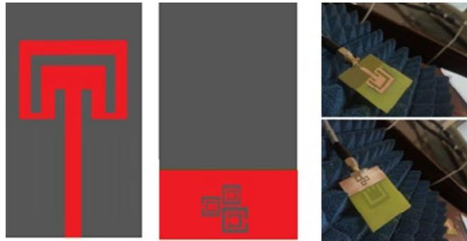
Fig. 9. The inverted U-shaped antenna with the three CSRR cells and their prototype
