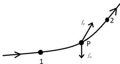
**Figure 1:** A fluid flows in a streamline. The points 1 and 2 are fixed in the same streamline. The point  $P$  represents an element of the fluid that moves along the streamline. The vectors represent the two force densities in the element of fluid, weight density  $\vec{f}_w$  and pressure force density  $\vec{f}_p$ .
